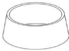
Thickness: 3mm Ceramic fibers 1200
