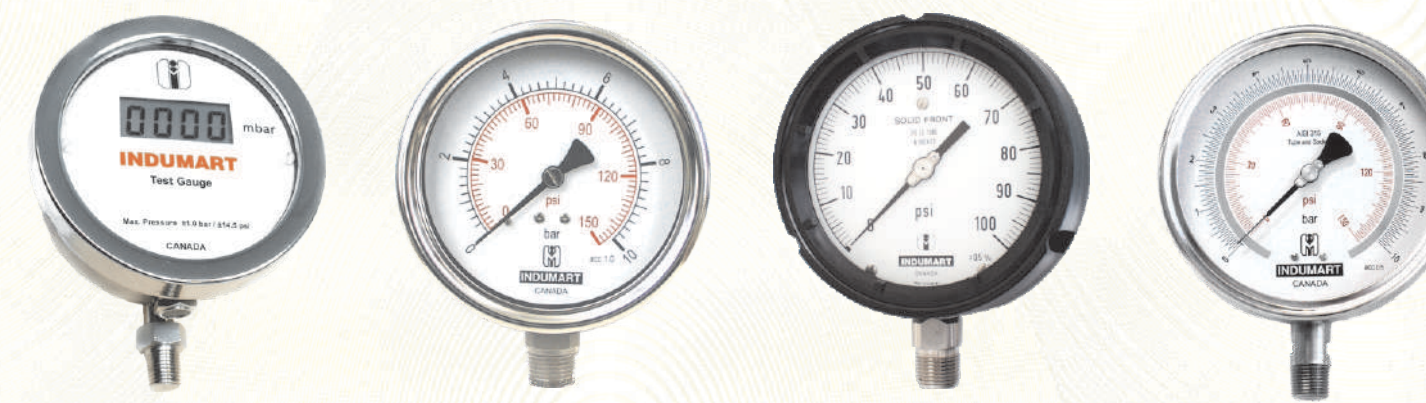
DIGITAL PRESSURE GAUGE 0.2% Accuracy Battery-operated Case: St. Steel Dial: 100 mm ALL ST. STEEL FILLABLE Dial: 50, 63, 80, 100 & 160 mm Range: Vac. & up to 60,000 psi SOLID FRONT GAUGE Case: Phenolic or St. Steel Full Blowout Back & Baffle Wall TEST PRESSURE GAUGE Accuracy: 0.5%, 0.25% & 0.1% Dial: 160mm mirrored scale
